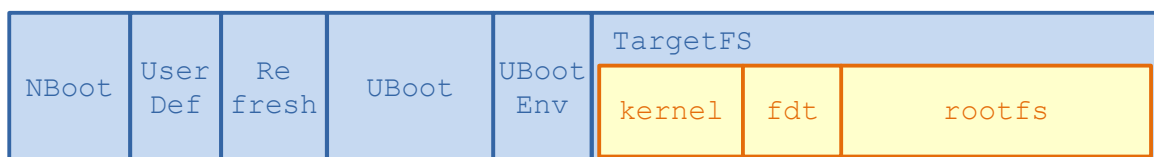
Figure 38: Linux kernel and device tree in separate UBI volumes
