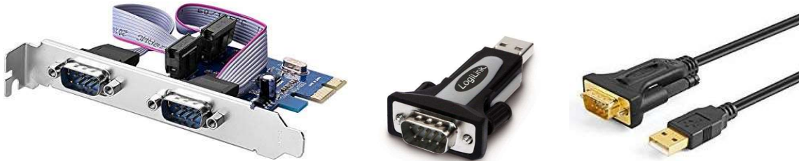
Figure 9: Serial port options for PCs without native port
